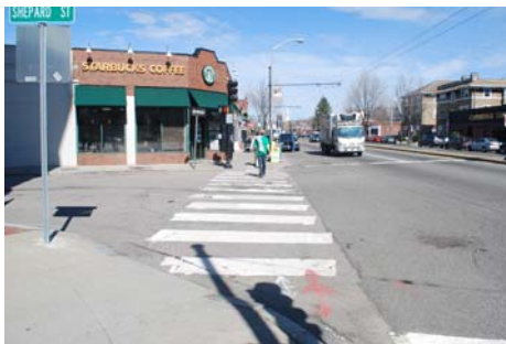
6. Proposed Garfield Street Crosswalk Cambridge has begun studying a pedestrian-automated crosswalk with bump-out curbs at Garfield Street. The painted lines show extent of projection. Additional, similar crosswalks are needed elsewhere on the Avenue.
