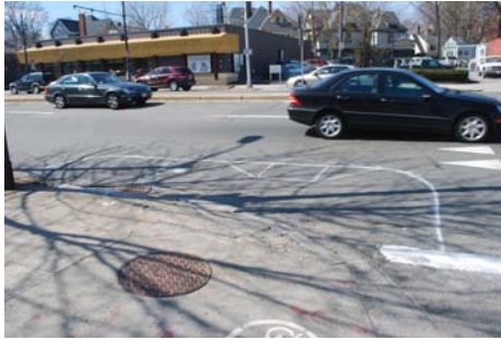
6. Proposed Garfield Street Crosswalk Cambridge has begun studying a pedestrian-automated crosswalk with bump-out curbs at Garfield Street. The painted lines show extent of projection. Additional, similar crosswalks are needed elsewhere on the Avenue.
